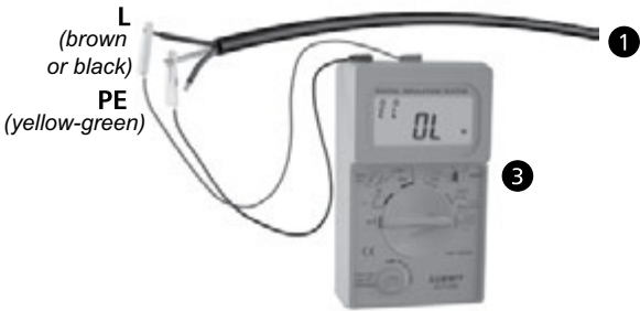
Insulation's resistance measurement
